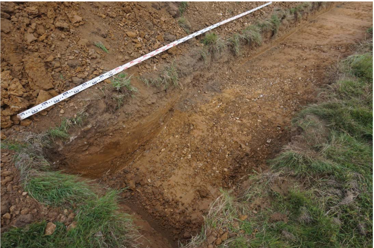
Plate 4: Looking NW at test pit located at S end of trench 1. The test pit was cutting into geological deposits of clay inter-bedded with flint gravel.
